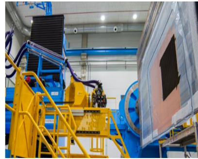
Figure 8. MTorres Dry Fiber Placement machine (DFP)
