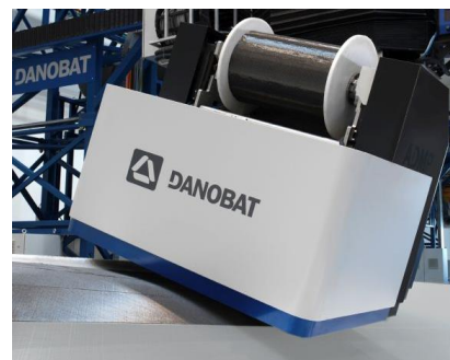
Figure 10. Danobat Automated Dry Material Placement machine (ADMP)
