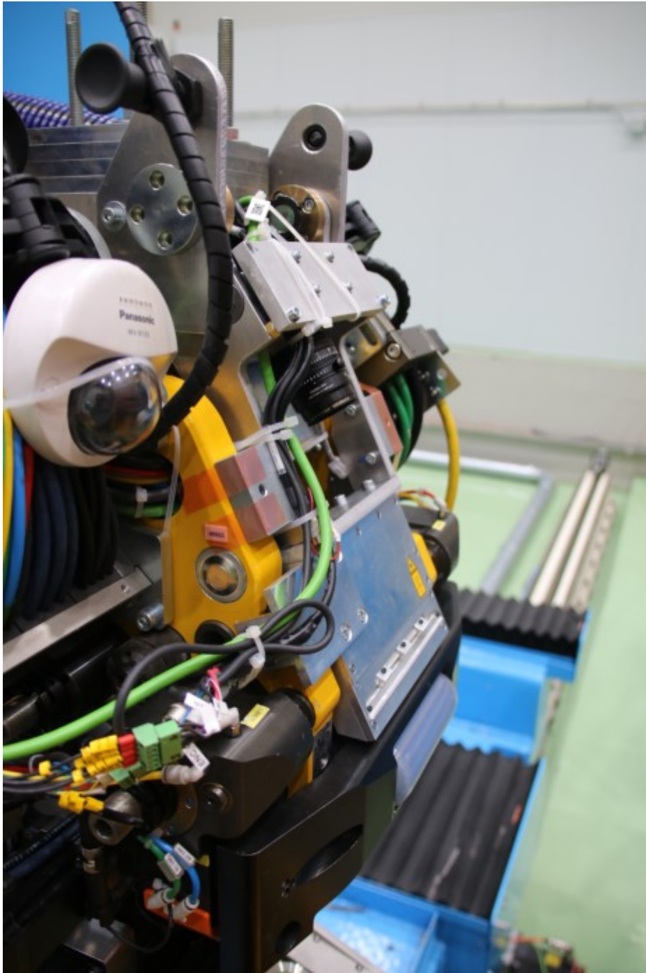
Sensor system for monitoring of the lay-up process with automated fiber placement (AFP).
